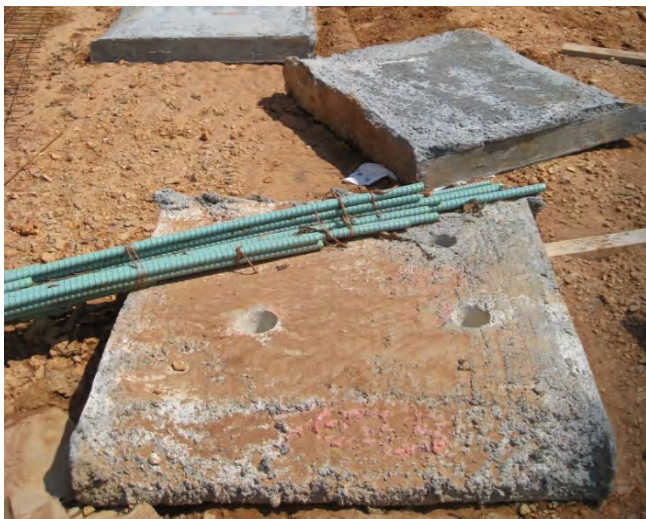
Figure 3.10: Photo. Curing of a shotcrete test panel on site. Photograph courtesy of Schnabel Engineering.
