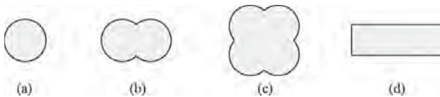
Figure 8.30 Shapes of deep mixed columns or walls: (a) circular, (b) dual, (c) quadral, and (d) panel.
