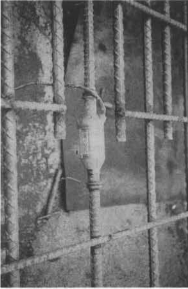
Figure 12.24 Rebar stress meter on a steel cage.
