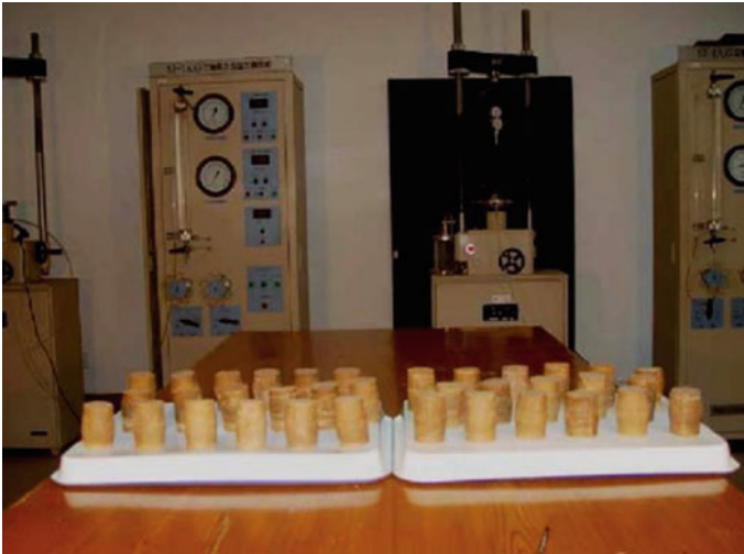
Fig. 6.12 Partial specimens after failure
