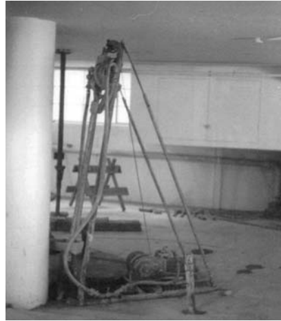
FIGURE 10.21 Pneumatically powered drill head mounted on lightweight frame.
