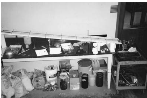
FIGURE 4.4 Tubing attached to a slant board for grout evaluation.
