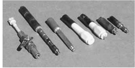
FIGURE 17.4 A variety of small packers are available for injection ports.
