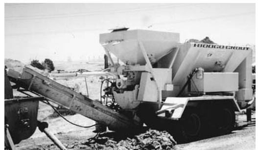
FIGURE 33.9 Typical volumetric batcher/mixer for concrete.
