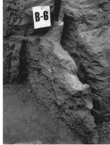
FIGURE 2.12 Two-winged grout mass resulting from hydraulic fracturing of the soil. (From Warner et al., 1992).
