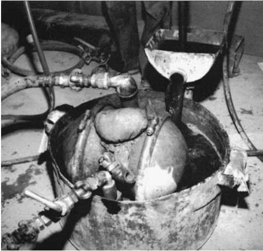
FIGURE 10.31 Collection device used to direct circulation return to mud tank.
