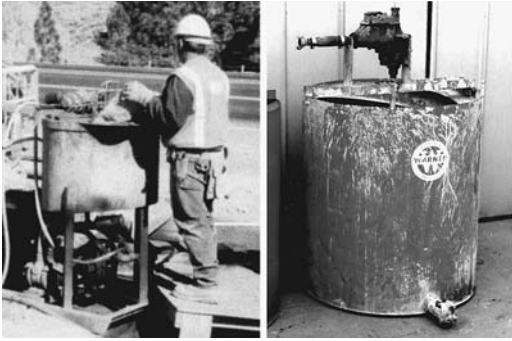
FIGURE 33.3 Ordinary paddle mixer (left) and high-speed mixer with downward inclined fins (right).
