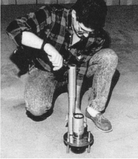
FIGURE 8.12 Typical pullout device for direct tension test.
