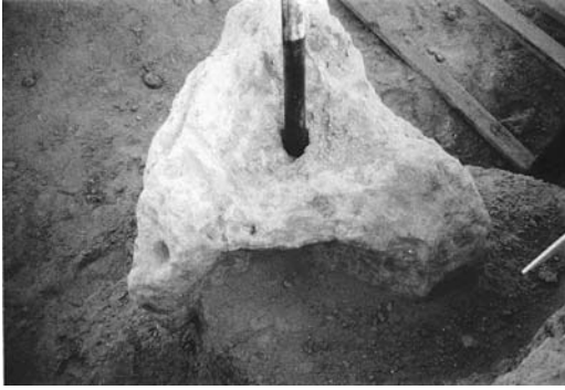
FIGURE 2.14 Globular D grout mass has low travel index.
