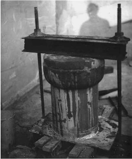
FIGURE 8.9 Test setup for expansive grouts.
