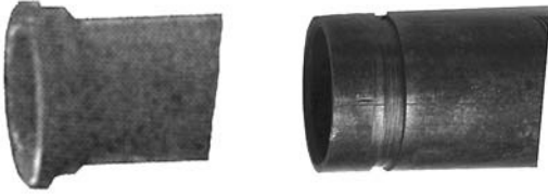
FIGURE 35.3 Heavy-duty weld end on left and conventional groove on right.
