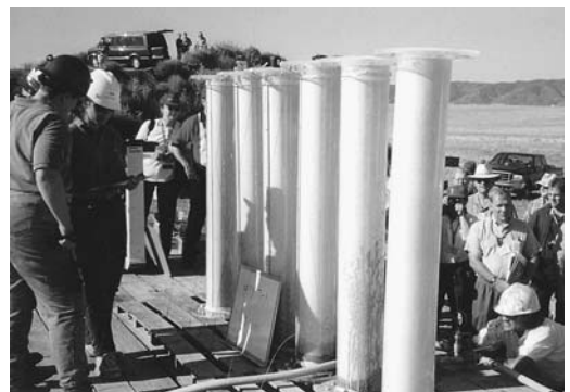
FIGURE 5.9 Sand-filled columns used for evaluation of ultrafine cement grouts.
