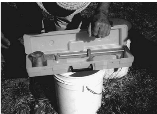
FIGURE 8.3 Baroid mud balance used to determine the specific gravity of grout.
