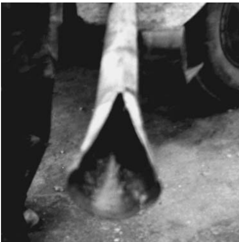
FIGURE 19.7 Weakening by scoring at a single location prior to the blast results in a belled casing.
