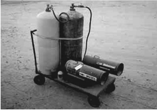
FIGURE 18.7 Highly portable propane-fueled heaters and tanks.
