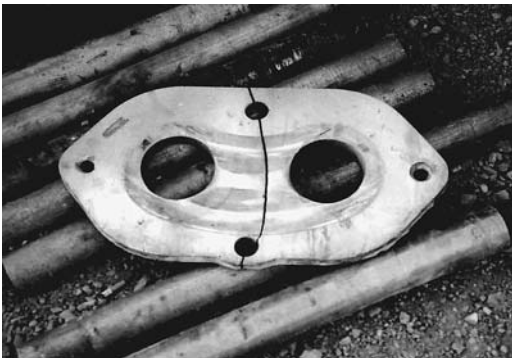
FIGURE 28.3 Excessively worn wear plate was broken in two.
