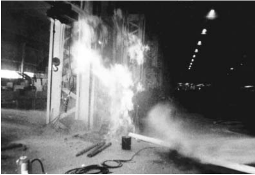
FIGURE 19.16 Explosion-engulfed drill rig on fire.
