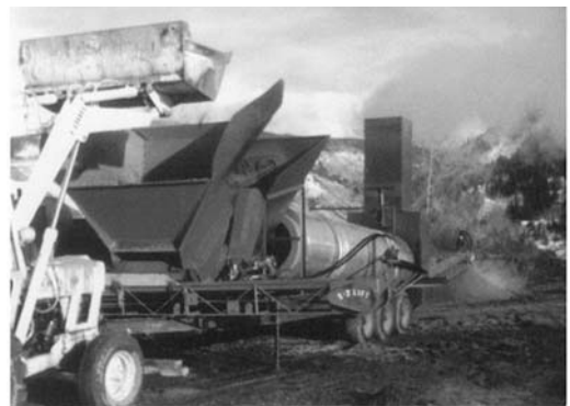
FIGURE 18.8 Portable drum kiln used to heat and dry fine-grained aggregate.
