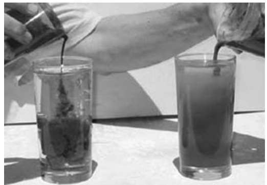
FIGURE 5.14 Identical grouts with and without viscosity-modifying antiwashout admixture.
