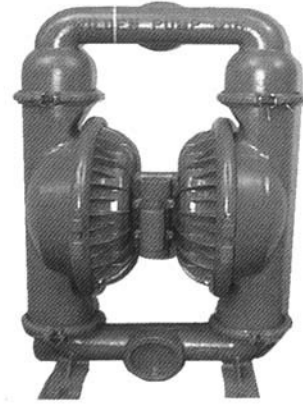
FIGURE 31.9 Duplex pneumatic diaphragm pump is cycled by compressed air against the internal diaphragm.
