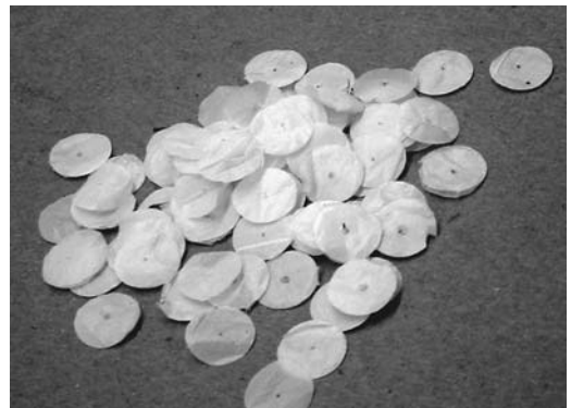
FIGURE 5.19 Plastic film punchings provide a good blocking material.
