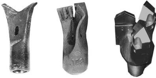
FIGURE 30.18 Drag bits: single piece, two and three blade on left, replaceable blade on right.
