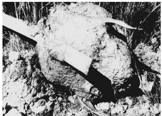
FIGURE 19.9 Four-leaf expanded pile base extricated from the soil by excavation.
