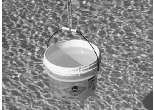
FIGURE 17.2 Bucket test to determine the water lost to evaporation.
