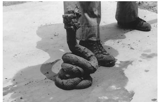
FIGURE 2.8 Stiff, mortarlike, low-mobility grout pumped from hose.
