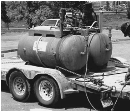
FIGURE 6.13 Foam generator used to develop prefoam, which will be fed into a mixer.
