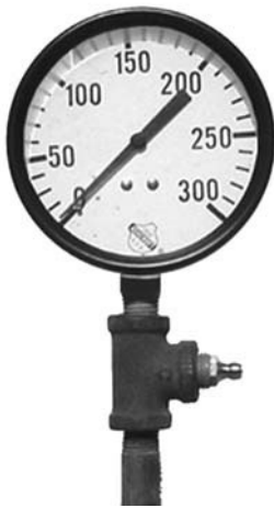
FIGURE 36.2 Zerk fitting on right is used to keep the gauge and the mounting nipple full of grease.
