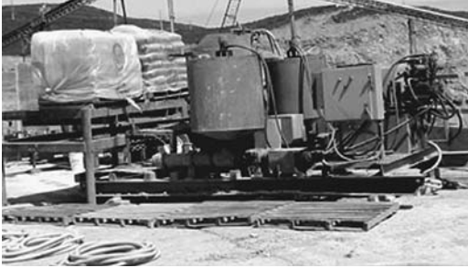
FIGURE 12.21 Highly portable skid-mounted grout plant.
