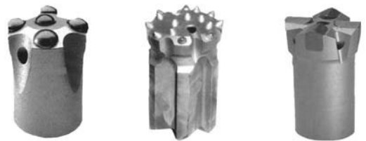
FIGURE 30.21 Heavy percussion bits: button on left, ballistic center, and four bladed on right.
