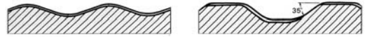
FIGURE 30.17 Heavy percussion rod threads, standard rope (R) on top, trapezoidal (T) on bottom.
