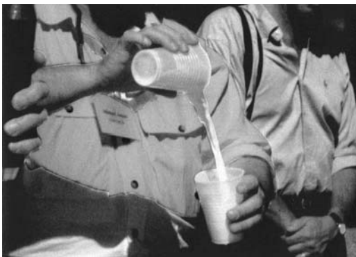
FIGURE 3.2 Tongue of grout gelled while being poured between two cups.
