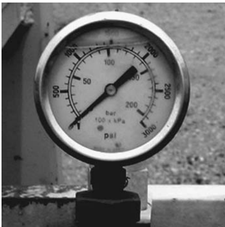
FIGURE 9.4 Gauges that display dual scales in both psi and bars are useful.
