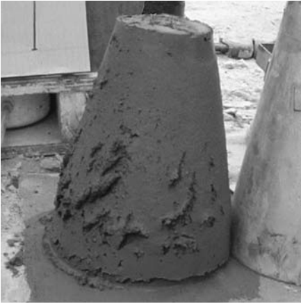
FIGURE 8.7 Voids and tears in lower portions of test specimen.
