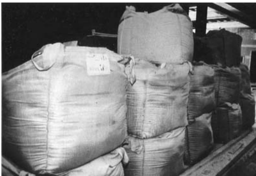
FIGURE 6.3 Bulk bin bags of preblended grout mix.
