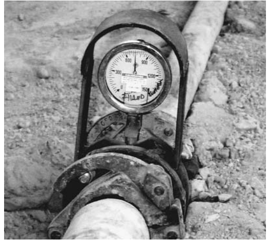
FIGURE 36.1 Gauge dial protective guards can be heavy and bulky.
