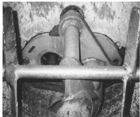
FIGURE 31.6 S-tube valve hugs wear plate with tight tolerance as it reciprocates between pump cylinders.
