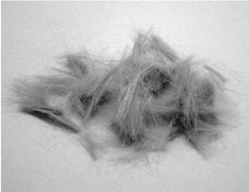
FIGURE 5.18 Fibrillated fibers form an interconnected random network.
