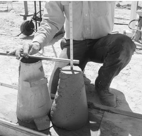
FIGURE 8.6 ASTM C 143 slump test.
