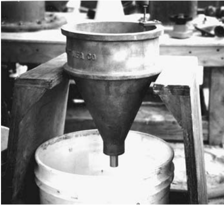
FIGURE 8.1 ASTM C 939 flow cone used to evaluate the flow properties of grout.
