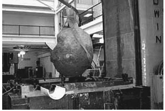
FIGURE 2.19 Grout mass being extricated from soil box in testing machine.
