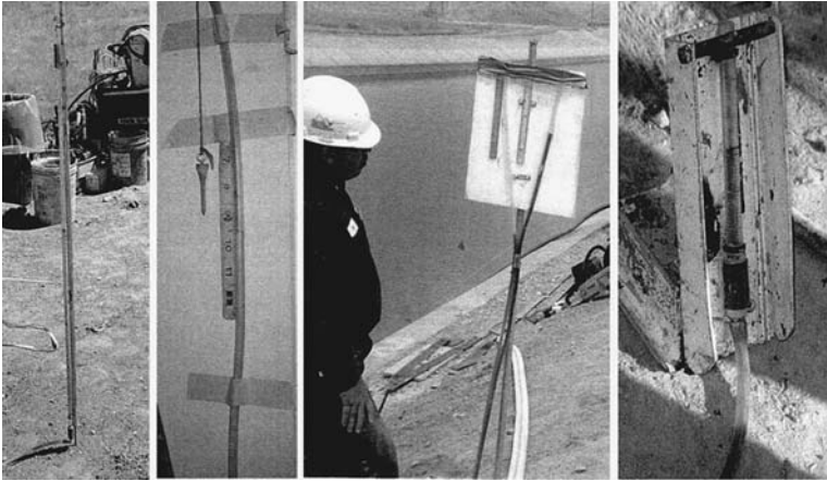
FIGURE 25.2 Variety of mountings for monometer terminals.
