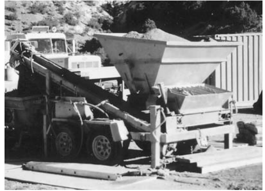
FIGURE 33.8 Typical batching/mixer for shotcrete.
