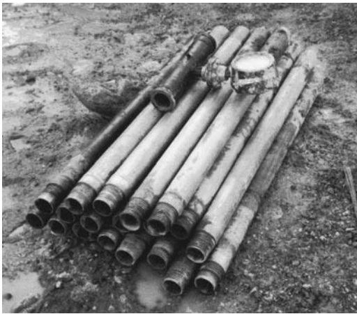
FIGURE 30.12 Heavy flush-walled robust casing used for compaction grouting.
