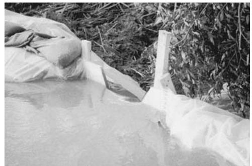
FIGURE 20.5 A standard V-shape weir to measure the flow rate.
