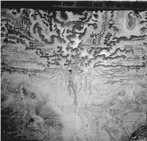
FIGURE 6.5 Test No. 5 grout dispersion.
