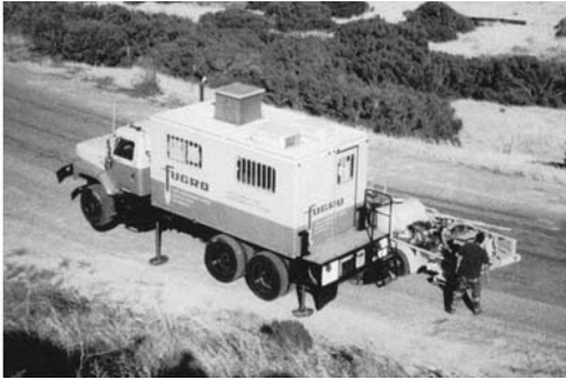
FIGURE 22.3 Large CPT rigs can setup and probe rapidly.
